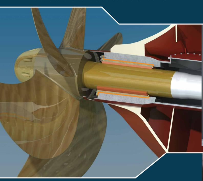
COMPAC SEAWATER LUBRICATED PROPELLER SHAFT BEARING SYSTEM
